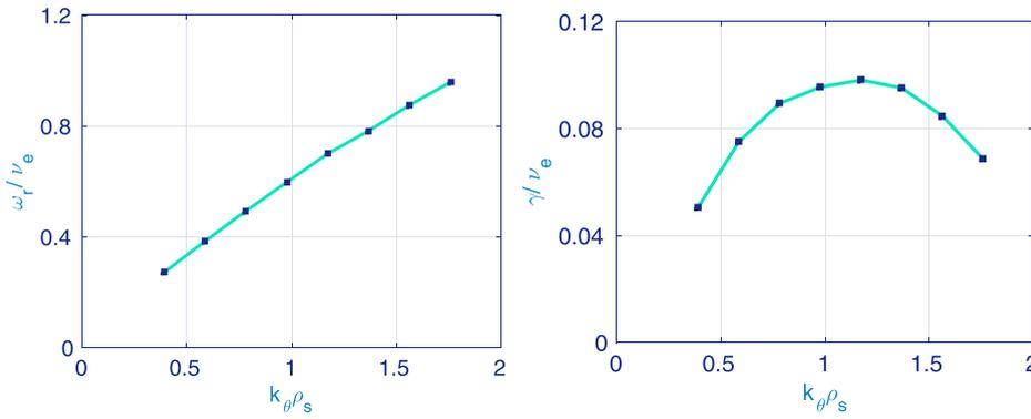
FIG. 13. Real frequency (left) and growth rate (right) with respect to  $k_\theta \rho_s$ .
