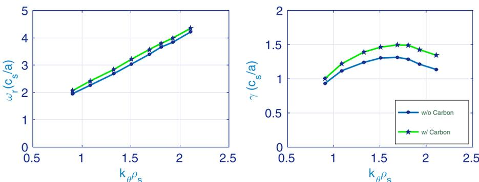
FIG. 10. Real frequency (left) and growth rate (right) vs  $k_\theta \rho_s$  at  $r/a = 0.93$ , with and without Carbon impurity.
