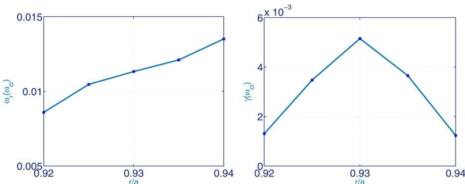
FIG. 1. Real frequency (left) and growth rate (right) vs radial location near edge for  $k_{\theta}\rho_s \approx 1.5$ .
