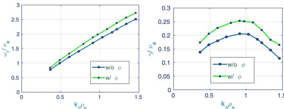
FIG. 20. Real frequency (left) and growth rate (right) with respect to  $k_\theta \rho_s$  with and without  $\tilde{\phi}$ .
