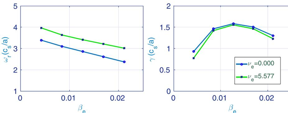
FIG. 5. Real frequency (left) and growth rate (right) vs electron  $\beta$  at  $r/a = 0.93$  for  $\nu_e = 0.0$  and  $\nu_e = 5.577$  for  $k_\theta \rho_s \simeq 1.5$ .
