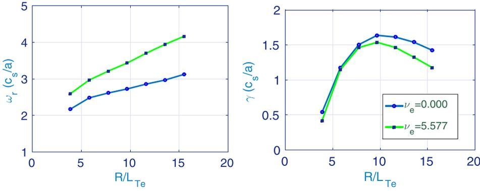
FIG. 4. Real frequency (left) and growth rate (right) vs electron temperature gradient at  $r/a = 0.93$  for  $\nu_e = 0.0$  and  $\nu_e = 5.577$  for  $k_\theta \rho_s \simeq 1.5$ .
