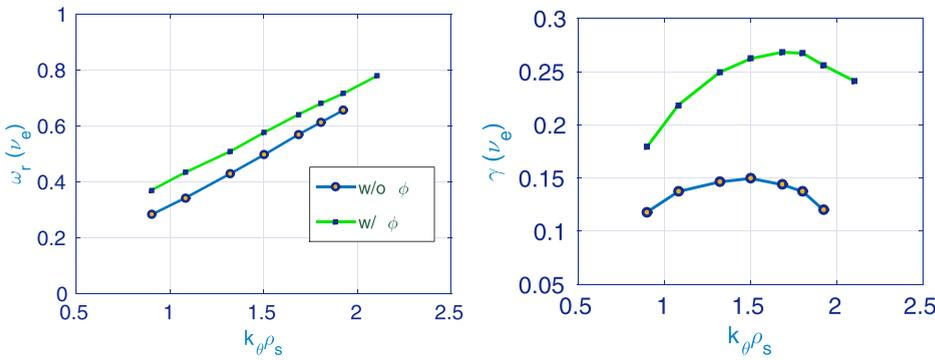
FIG. 11. Real frequency (left) and growth rate (right) vs  $k_0 \rho_s$  at  $r/a = 0.93$ , with and without the electrostatic potential  $\tilde{\phi}$ .
