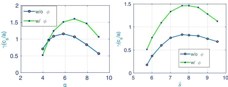
FIG. 12. Growth rate vs  $q$  (left) and shear  $\hat{s}$  (right) at  $k_0 \rho_s = 1.5$ , with and without electrostatic potential  $\tilde{\phi}$ .
