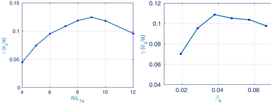
FIG. 18. Growth rates as a function of electron temperature gradient (left) and  $\beta_e$  (right) for  $k_\theta \rho_s \simeq 0.9$ .
