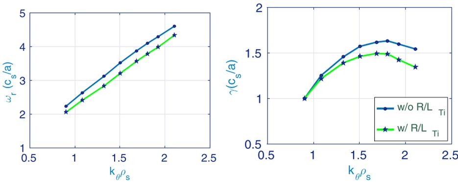
FIG. 9. Real frequency (left) and growth rate (right) vs  $k_\theta \rho_s$  at  $r/a = 0.93$ , with and without ion temperature gradient.
