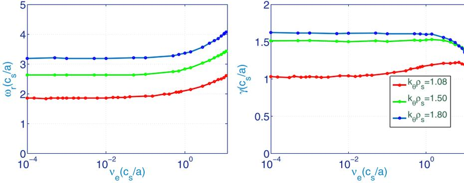
FIG. 2. Real frequency (left) and growth rate (right) vs collision frequency at  $r/a = 0.93$  for  $k_\theta \rho_s = 1.08, 1.5$ , and  $1.8$ .
